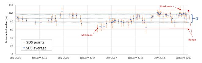
**Figure 6.** This figure represents, at one sampling location (see Figure 3, C section), the distances between the baseline and the points that compose each SDS (points in light orange, considering a 100 m buffer), as well as their average blue point). The proxy standard deviation (9.8 m, dashed line in blue) was derived considering all SDS average distances while the range (45.1 m, solid line in red) was defined as the difference between the furthest SDS (107.7 m) and the closest one (63.7 m).
