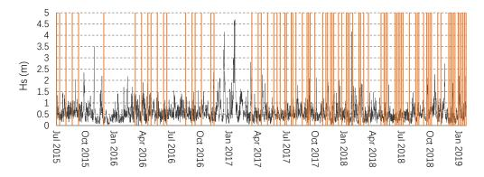
**Figure 2.** In black color, significant wave height (m) for the coastal segment around the Valencia Port (Spanish Port Authority, SIMAR point 2081114) along the study period (2015–2019). In orange, Sentinel-2 is considered for SDS extraction. The presence of clouds over the shore is the cause of data gaps, forcing use of a slightly smaller quantity of images at certain segments.
