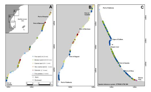
**Figure 3.** Sampling locations along the Gulf of Valencia, which appears divided from north to south in three sectors (A–C). Grain sizes of the beaches (as  $D_{50}$ ) are represented by different colors and the morphological classification by symbols (circles and crosses for open and enclosed beaches respectively). The black arrow identifies the site used in Figure 6 for describing the definition of SDS variability.
