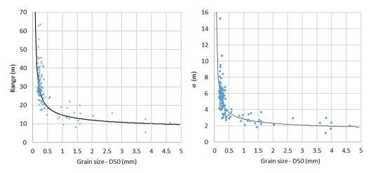
**Figure 9.** Shoreline variability as a function of sediment grain size. On the left, the relationship is defined for 100 m buffers by the equation: range =  $1/(0.0675 + 0.0234*\ln(D_{50}))$ . On the right, for 200 m buffers,  $\sigma = 1/(0.3522 + 0.1143*\ln(D_{50}))$ .
