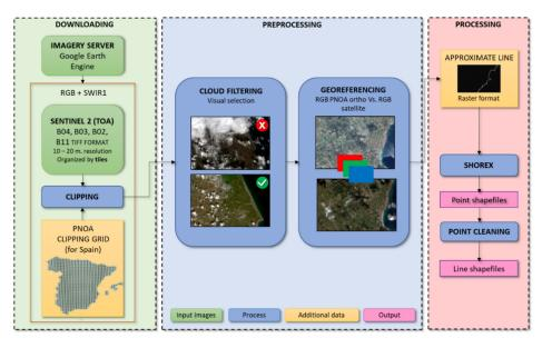
**Figure 4.** SHOREX workflow and its three main phases: downloading (**left**), preprocessing (**middle**), and processing (**right**).
