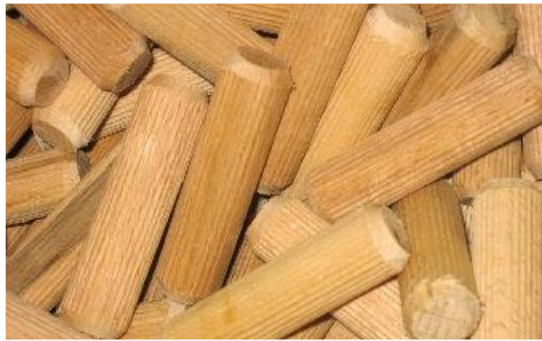
Illustration 49: Wood dowel pins
