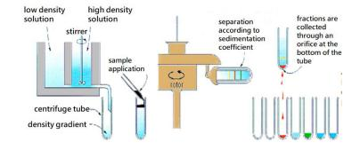
**Figure 6.** Stages of rate-zonal centrifugation. (A) Creation of a density gradient with an automatic device (B) Placing the sample on the gradient at the top of the tube (C) placing the tubes in the swinging-bucket rotor and centrifugation (D) collecting the pellets separated in bands (Source: Técnicas de laboratorio en bioquímica. Centrifugación. <u>http://biomodel.uah.es/</u>).
