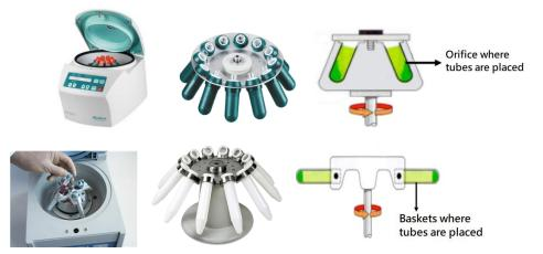
**Figure 2.** Upper raw: fixed-angle centrifuge, components and tubes position during spinning. Bottom row: swinging head centrifuge, components and tubes position during spinning.
