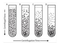
Figure 3. Differential centrifugation (Mark Frei, BioFiles).
