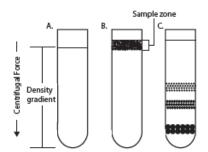
Figure 5. Rate-zonal centrifugation (Biofiles online. Sigma.com/biofiles)
