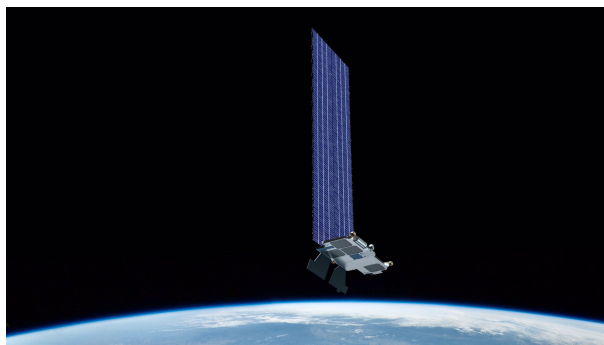
Figure 13: Starlink L1-1 satellite[15]
