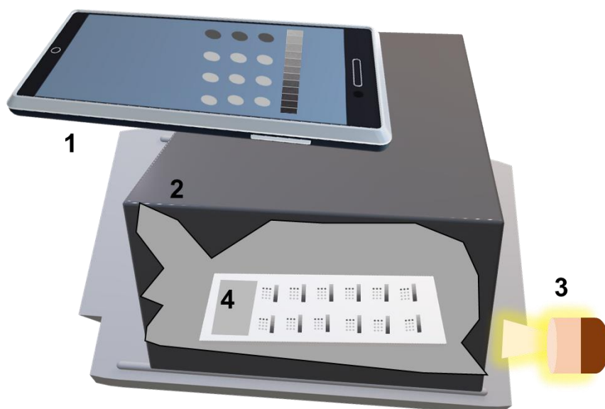
Figure SI.5. Assembly for the smartphone-based detection of HCR products. (1) Smartphone for detection (iPhone 11 Pro). (2) Homemade capture chamber (9×11.5×8 cm). The top layer had a 3×3 cm central window that fitted the protruding camera. The bottom was a translucent platform where the chip was located. (3) Illumination 5 W flash LED, e.g., smartphone torch. (4) Hybridization polycarbonate chip. A color palette is included and placed close to all the arrays to correct variations in illumination.
