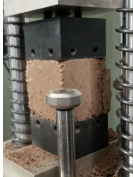
Fig. 4.1-3 A cubic specimen in a compressive strength test.
