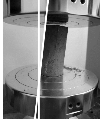
Fig. 4.1-2 Cylindrical specimen deformed when unmolding by sample plasticity.
