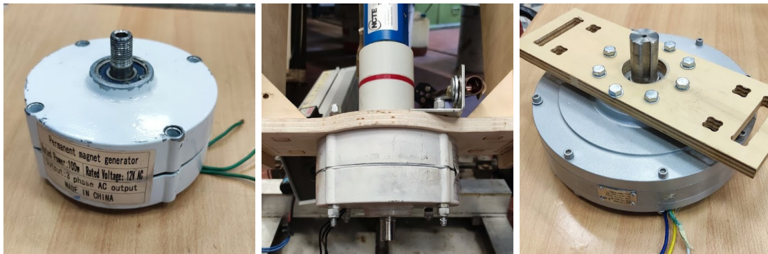
(a) Conventional PM generator of 100W (b) Conventional PM generator of 200W (mounted) (c) Coreless stator AFPM generator of 200W
