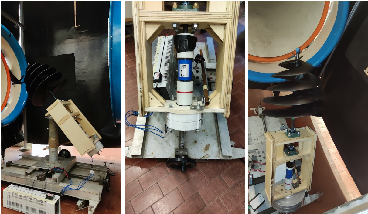
(a) General lay-out of electrical experience in wind tunnel (b) Inner of the wooden support box with conventional generator (white color) (c) Measurements with coreless stator AFPM generator of 200W (grey color)
