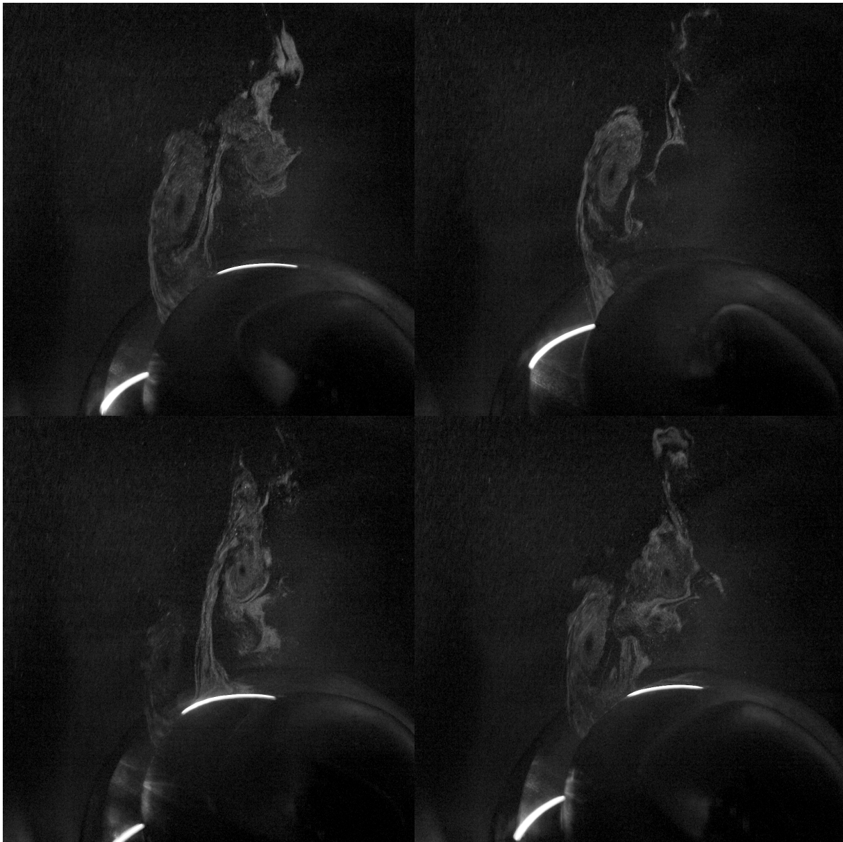
Figure 5.25: Image acquisition, representation of one revolution for horizontal plane with 20 degree and 10m/s configuration
