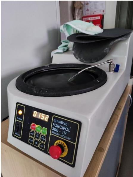
Figure 22 - Sanding-polishing machine
