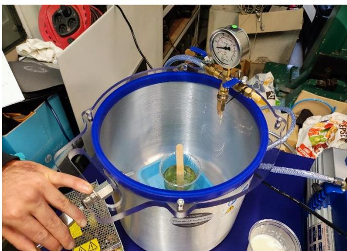
Figure 16 - Vacuum chamber 1
