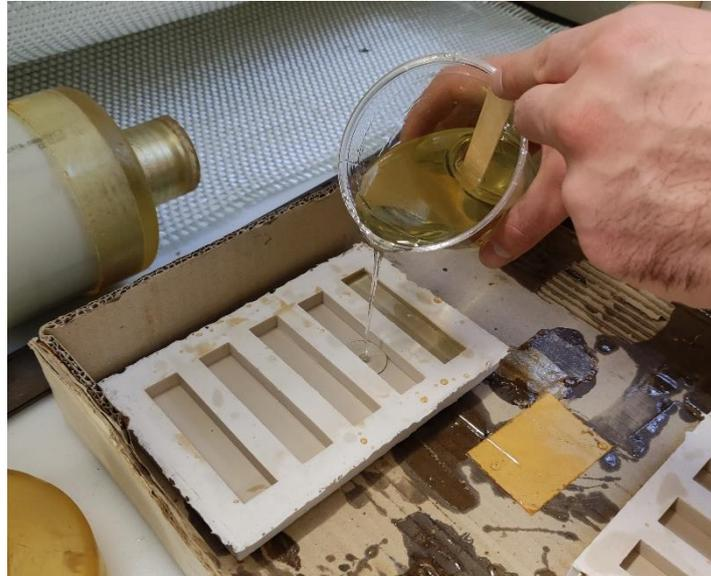
Figure 11 - Samples mould
