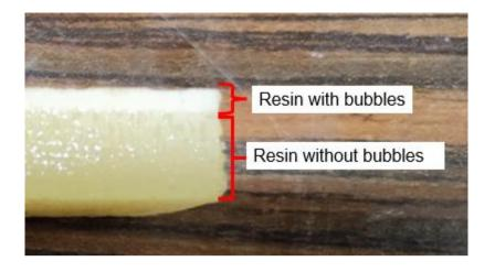
Figure 19 - Sample of resin with flame retardant
