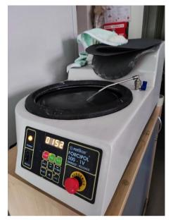
Figure 22 - Sanding-polishing machine
