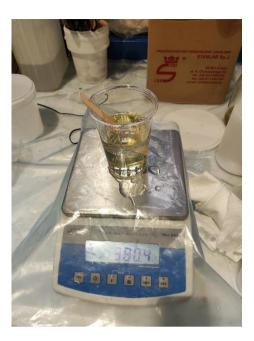
Figure 12 - Glass with resin in the scale
