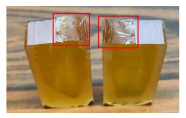
Figure 24 - Crack lenght(sample without flame retardant)
