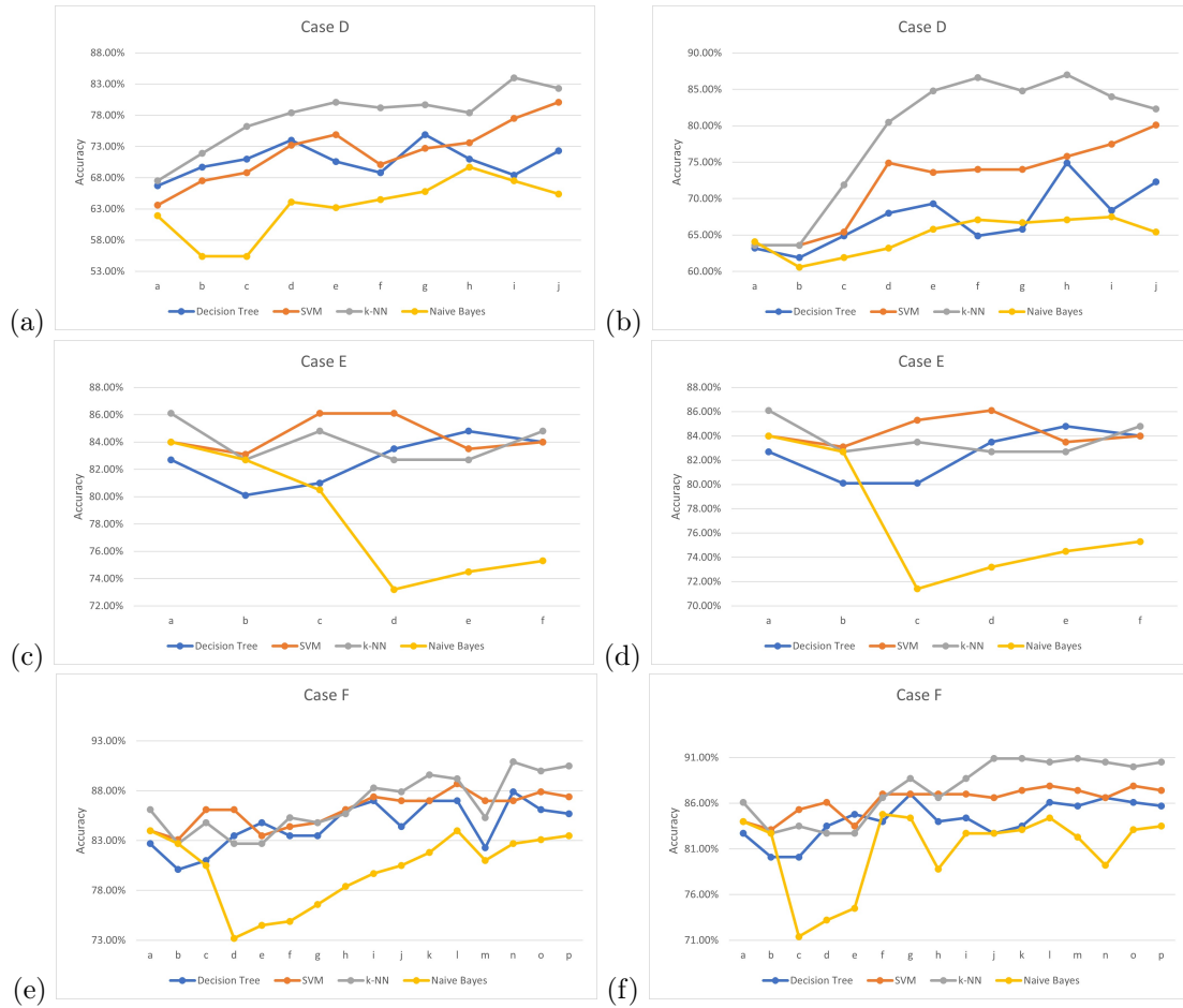
Figure 15: Line graphs of cases D, E & F. Plots (a), (c) & (e) represent cases ordered by the one-way ANOVA ranking. Plots (b), (d) & (f) represent cases ordered by the Kruskal-Wallis test ranking.
