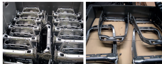
Figure 6. Improvement in placement of main structures inside the “box pallet”. Initial situation (left) and improved situation (right) (source: authors).
