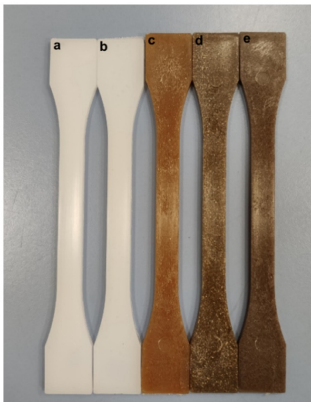
Figure III.1.8. Visual appearance of the samples: (a) BioHDPE; (b) BioHDPE/PE-g-MA; (c) BioHDPE/Hemp/PE-g-MA; (d) BioHDPE/Flax/PE-g-MA; (e) BioHDPE/Jute/PE-g-MA.
