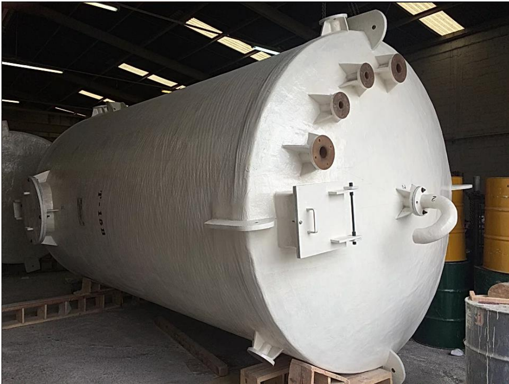
Figure 11 Tank for store corrosive elements
