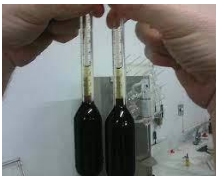
Fig 13. Determination of fat content using butyrometer
