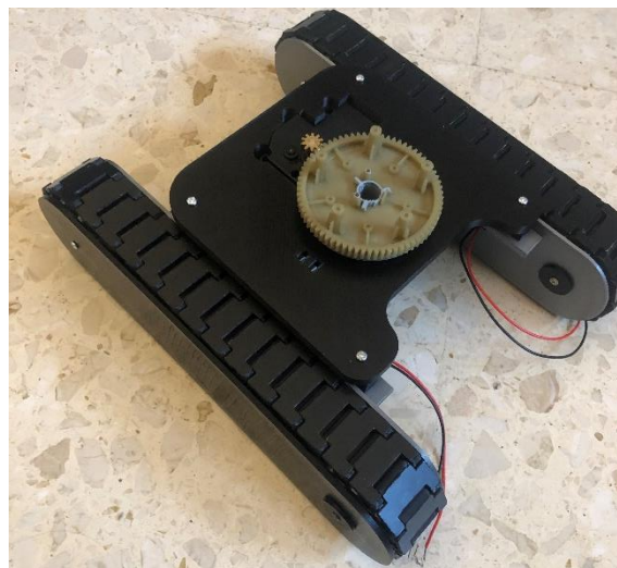
Figure 30: Assembled base plate including tracks, rotational gear + lock, and rotational motor
