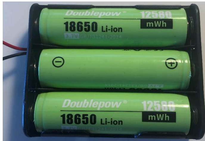
Figure 8: 18650 Li-ion batteries in the holder connected in series
