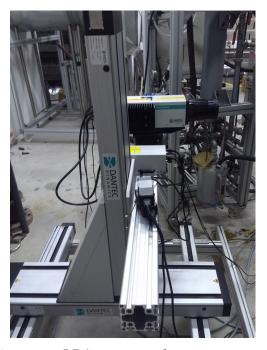
Figure 3.7: LDA system and traverse system.
