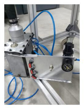
Figure 3.8: Seed particles generator.
