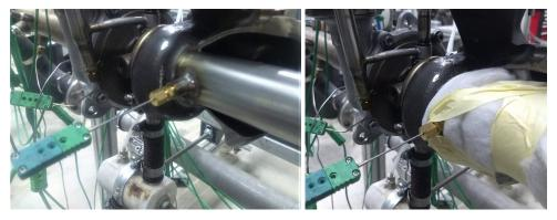
(a) New rotor outlet pipe.
