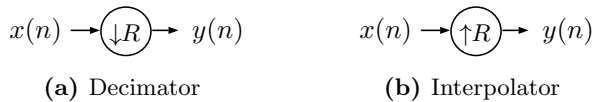
Figure 4.1: Block diagram of a decimator and an interpolator in (a) and (b), respectively.
