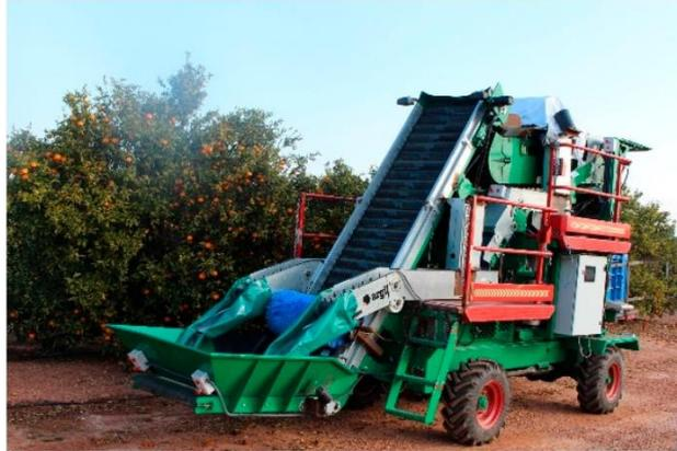
Figure 1. Prototype of a self-propelled harvest-assist platform.
