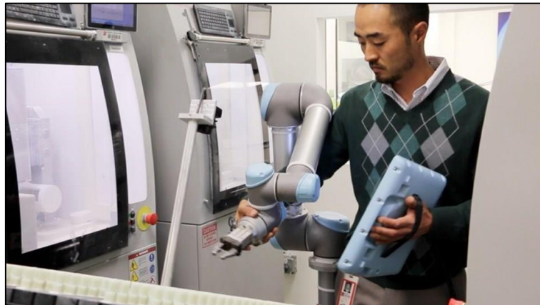
Figure 2: Universal Robot Hand Guide function
