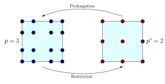
Figure 1: Restriction and prolongation operator of a element associated with degree p = 3 and  $p^* = 2$  in the FEM.
