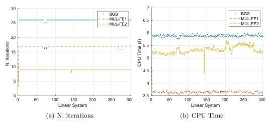
Figure 2: Comparison of the multilevel preconditioner where the second level is obtained from  $p_* = 1$  (MUL-FE1) and  $p_* = 2$  (MUL-FE2), and the BGS preconditioner for the solution of the time-dependent SP<sub>1</sub> equations.
