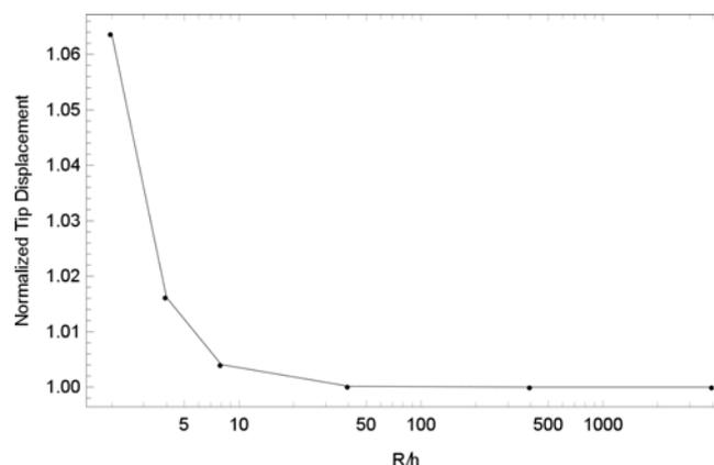
**Figure 2:** Quarter-Circular Cantilver Uniform Beam Under a Shear Force at its Free End - Shear and Membrane Locking Tests
