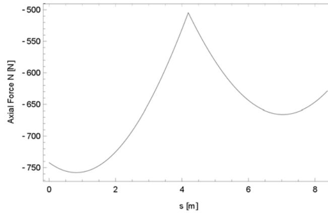
**Figure 5:** Clamped-Clamped Circular Tapered Beam with Tip Load - Axial Force Diagram
