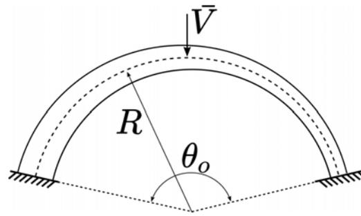
**Figure 4:** Clamped-Clamped Circular Tapered Beam with Tip Load
