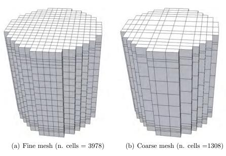
Figure 2: Meshes for NEACRP reactor.
