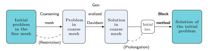
Figure 1: Scheme for the multilevel initialization.
