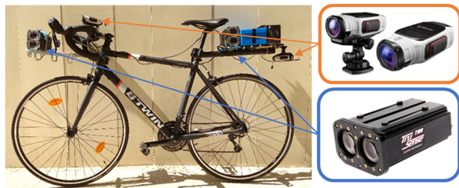
Figure 3. Instrumented bicycle equipped by cameras and a laser device.
