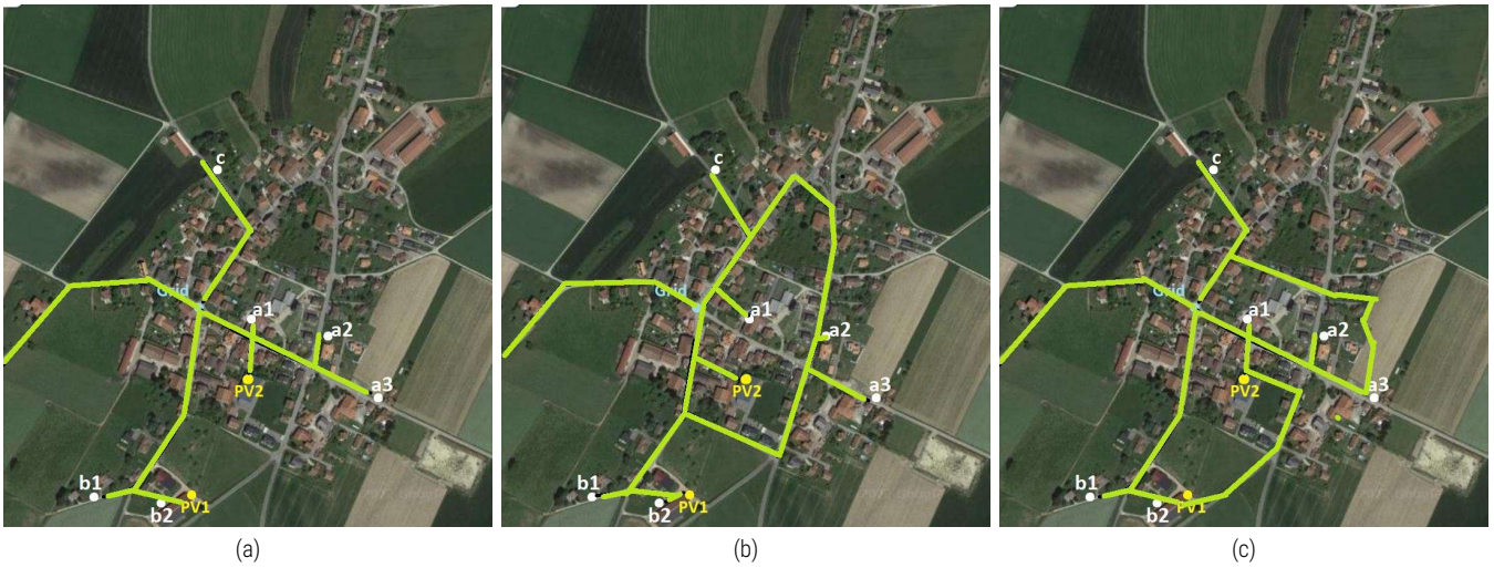
Fig. 3.3 Layout electrical lines for District case: (a) Radial Configuration; (b) Ring Configuration (c) Mesh Configuration.
