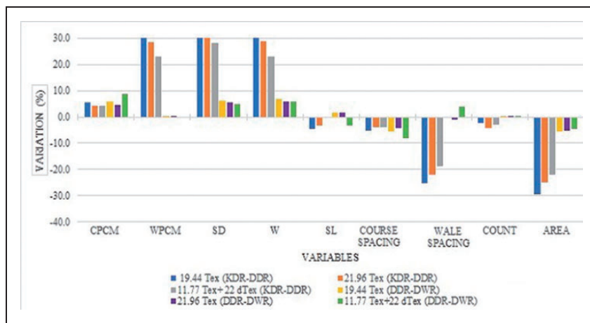
Figure 4. Dimensional variations as the percentages obtained from analyzing the three produced 1 × 1 rib structures, two of which with 19.44 and 21.96 Tex 100% cotton, and one with 11.77 Tex with half-plated 22 dTex elastane, between relaxation states KDR–DDR and DDR–DWR.
