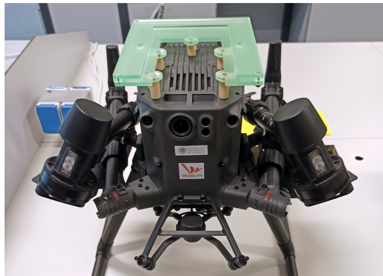
Figure 2. DJI Matrice 300 RTK fitted with upper cargo bay.
