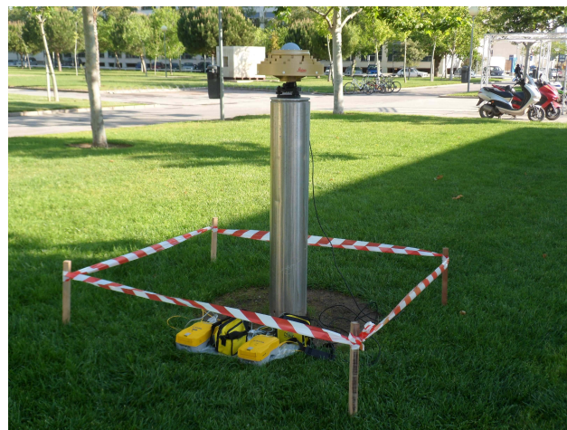
Figure 1. Global Navigation Satellite System (GNSS) measurement at the Universitat Politècnica de València (UPV) calibration baseline using a 3D choke-ring antenna equipped with a signal splitter and two receivers collecting the same signals.
