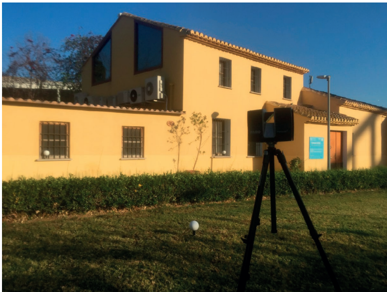
Figure 1. 3D laser scanner and placement of spheres in the farmhouse.
