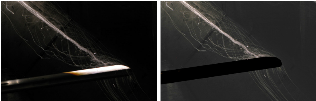
(a) Correct exposure of bubbles (b) Manipulated image to highlight vortex Figure 2.4: Wingtip vortex from a NACA0012 airfoil at 10 m/s [11]
