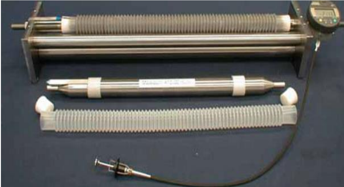
Figure21 Instruments used for autogenous shrinkage measurement [54].
