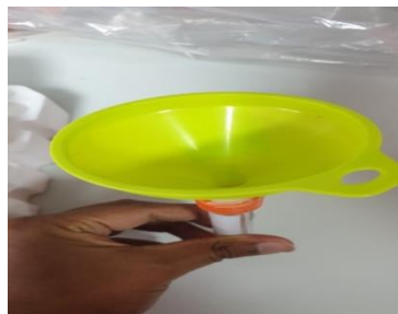
Fig. 12 The Funnel attached with the tube filled with 80% alcohol.
