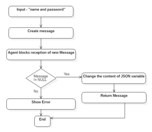
**Figure 9.** The logic of algorithm of sources input.
