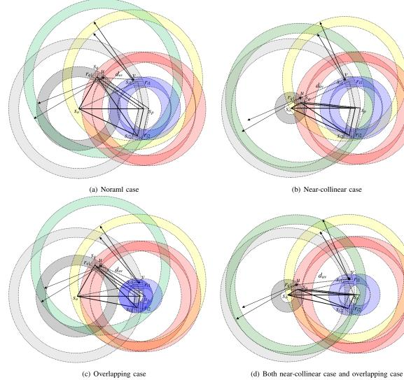
Fig. 3. Localization without flip ambiguities using trilateration.
