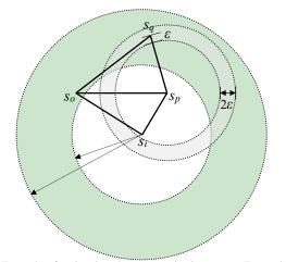
Fig. 1. Example of estimating the communication range. For node  $s_i$ , the minimum of the estimated communication range is  $\hat{d}_{io} - \varepsilon$ , and the maximum is  $\hat{d}_{pi} + \hat{d}_{pq} + 2\varepsilon$ .
