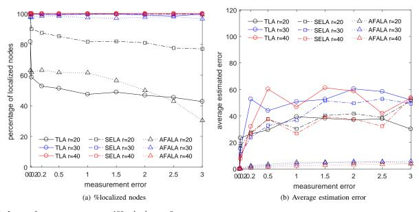
Fig. 6. Impact of measurement error. n = 100, s $\triangle$ ,  $d_{max} = 0$ .
