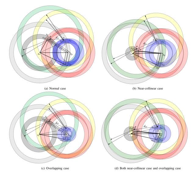
Fig. 2. Localization without flip ambiguities using bilateration.
