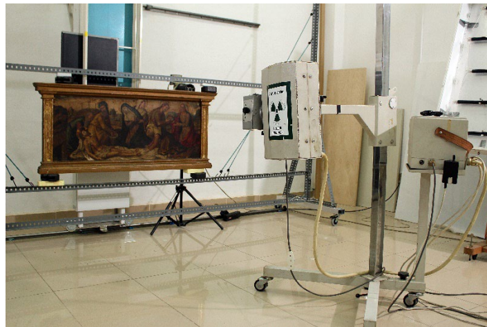
Fig. 2. The radiography set up.
