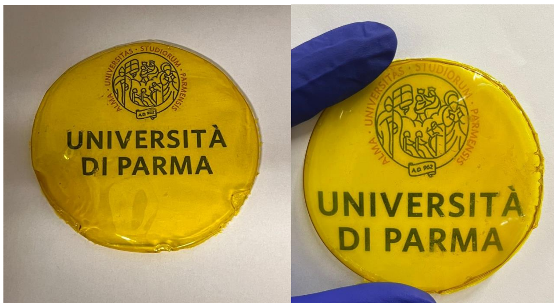
Figure 2: Photo of the PIM-1 film (left) and the crosslinked PIM-1 (right) films obtained.
