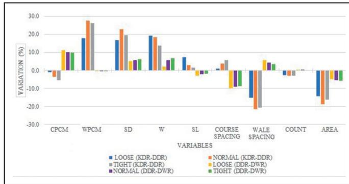
**Figure 2.** The dimensional variations as percentages obtained by analyzing the three interlock structures made with 19.44 Tex 100% cotton with loosely knitted loops (SL=0.360 cm), intermediately knitted loops (SL=0.340 cm) and tightly knitted loops (SL = 0.320 cm) between relaxation states KDR–DDR and DDR–DWR.
