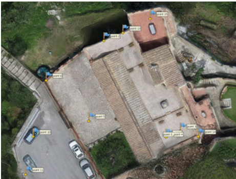
Fig. 7. Textured model of the villa in the software Agisoft Metashape , with the GCP used to link the two point clouds.
