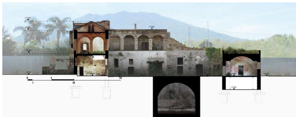
Fig. 4. A section on the courtyard of the masseria of the Duke of Salza. The section intercepts the cistern, along the shorter side, the room on the groundfloor where there was the scalandrone , a stable with the upper terrace, the meeting hall in the apartment of the administrator and the attic. On the background, there's the loggia facing the courtyard (Source: Author, 2018).
