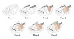
Fig. 4. Main construction phases of the block.
