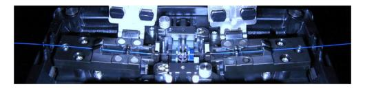
FIGURE 11 Fiber fusion splicer
