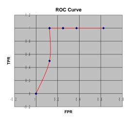
**Fig. 12** ROC curve of anomaly detection at S-Node 2 with different  $\delta_x$  values
