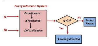
Fig. 7 Anomaly detection system at an A-Node
