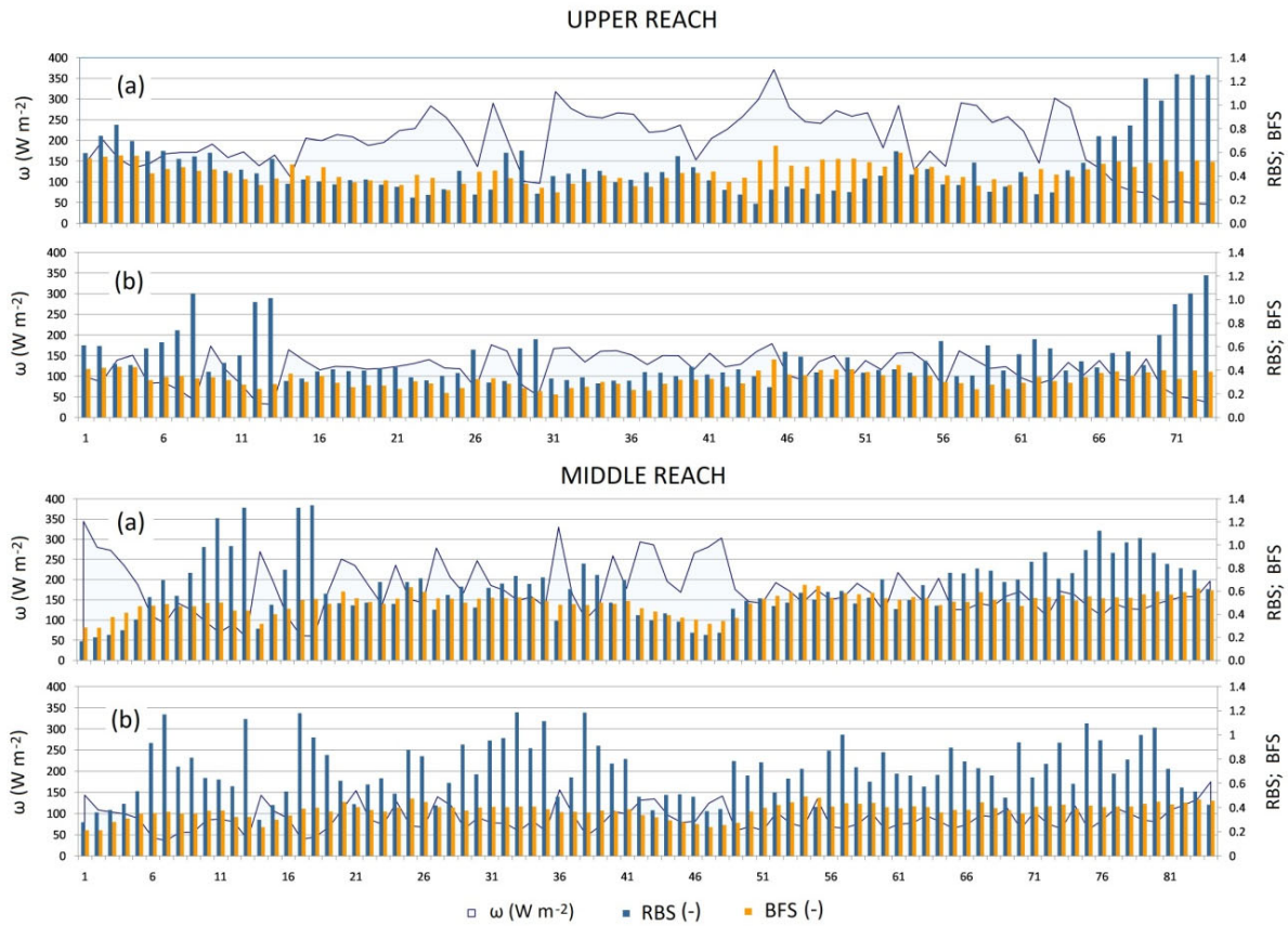
Figure 14. Mean stream power ( \omega ) versus the Relative Bed Stability (RBS) and Bed Form Stability (BFS) indices estimated in cross-sections along the upper and middle RCRs, in a downstream direction. Flow peaks of 19-20 April 2019 (a) and 12-13 September 2019 (b).
