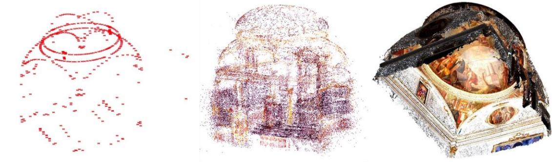
Figure 4. Cloud of 526 points from Camarín chapel taken with a total station (left). Dispersed point cloud (center) and point cloud with texture (right) of Camarín obtained with Photoscan program of Agisoft .
