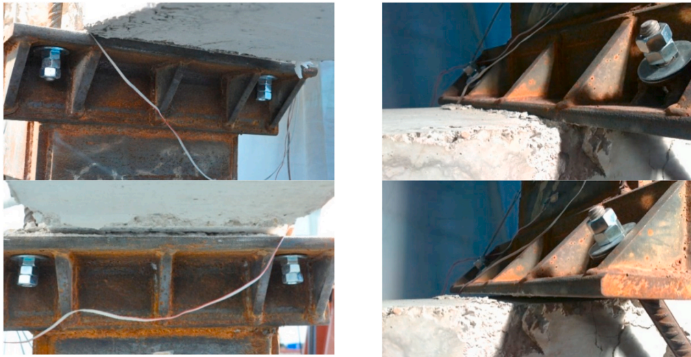
c. Contact and loss of contact of capitals in tension-compression reverse cycles.
