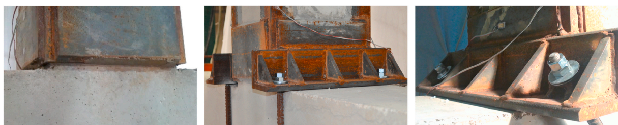
a. W typology. No connection. b. VB typology. Vertical bar. c. DB typology. Diagonal bar.
