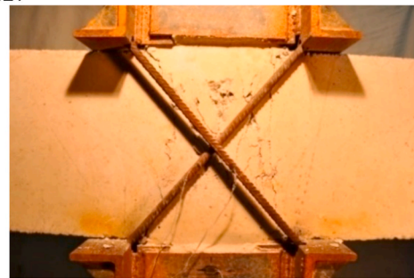
Fig. 7. Left: column shear force vs. drift ratio. Right: joint view at the 3.5% drift ratio in the specimens without axial loads (L0), and the 2.5% drift ratio in those with the axial load (L1).
