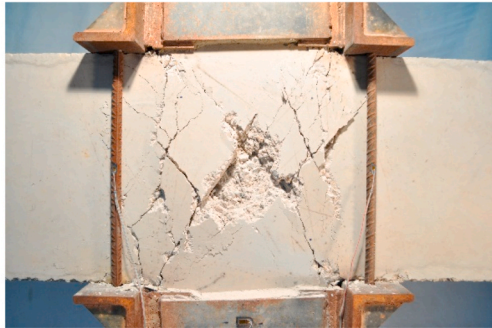
c. A.VB.L1 damage state after first cycle for the 3% drift ratio.
