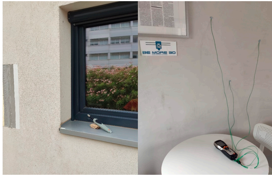
Figure 4. Thermal transmittance measurement process.
