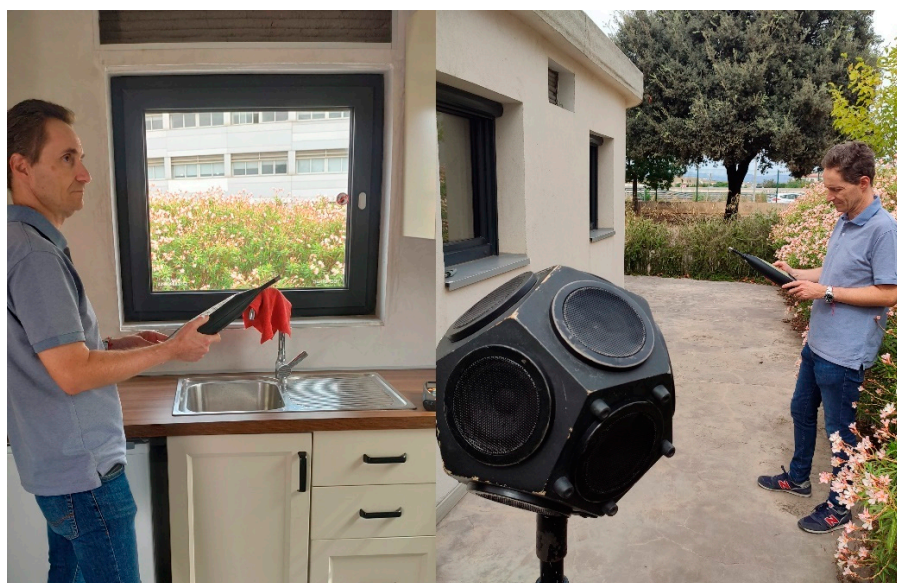
Figure 5. Sound reduction index measurement process.
