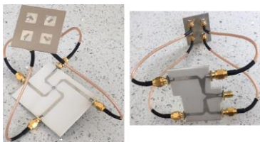
Fig. 7 Antenna array with feeding networks
