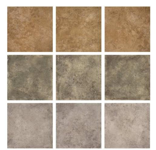
Figure 3.8: VxC TSG stone samples. From up to down; three samples of petra, santiago and somport models, each one corresponding to a different surface grade.
