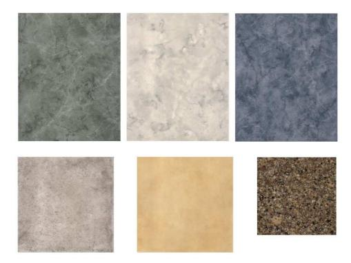
In order to study the temporal response we measured the mean CIE Lab colour of each piece. And also, in order to study spatial response we randomly oriented the pieces in each capture. The CIE Lab is a perceptually uniform colour space and we can measure the perceptual difference between two colours using the Euclidean distance in this space [33]. Thus, colour differences can be measured in a very similar way to the human perception of colours.
