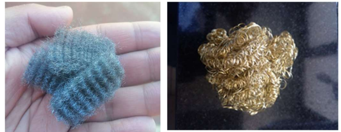
Figure 2. Aluminum and steel alloy fibers used in mixtures.
