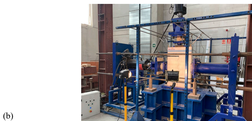
Figure 2. Experimental test setup for the dry joints subjected to combined axial, bending and shear forces: (a) sketch and (b) photo of setup.
