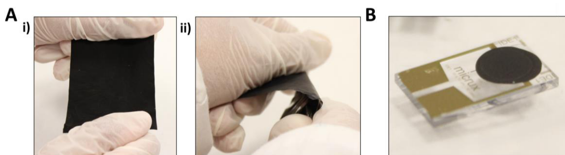
Figure 1. Chitosan-CB membrane configuration such as (A) self-standing membrane under (i) stretching and (ii) twisting, and (B) membrane integrated into miniaturized electrodes.
